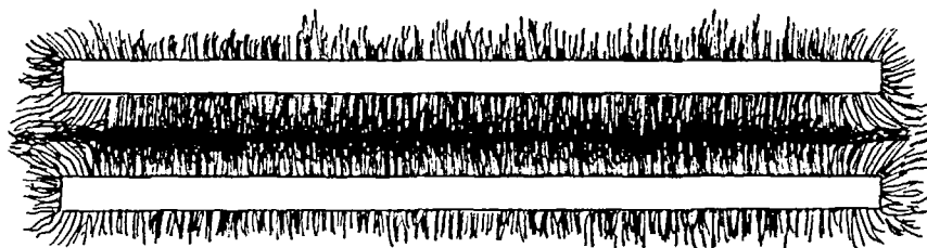
FIG. 9. Portrayal of the pattern of fluid flow adjacent to the surface of a slat.
